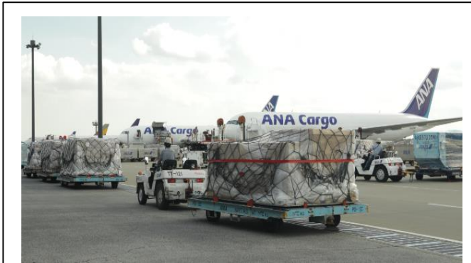
ULDs will be carried out from the warehouse on dollies
