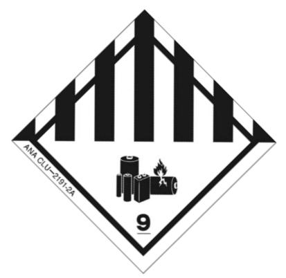
Minimum dimensions: 100mm x 100mm The line inside the edge forming the diamond: more than 2mm Symbol: seven vertical black stripes in upper half, battery group, one broken and emitting flame in lower half
