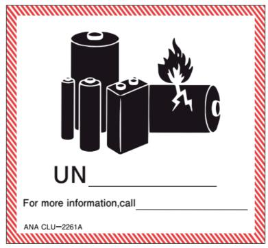
Minimum dimensions: 120 mm wide x 110 mm high Minimum width of the hatching: 5mm Hatching color: Red Symbol: group of batteries, one damaged and emitting flame,
